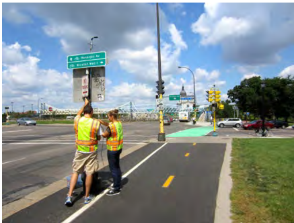
Figure 2-8: A contractor setting up a camera at the colored crosswalk markings
