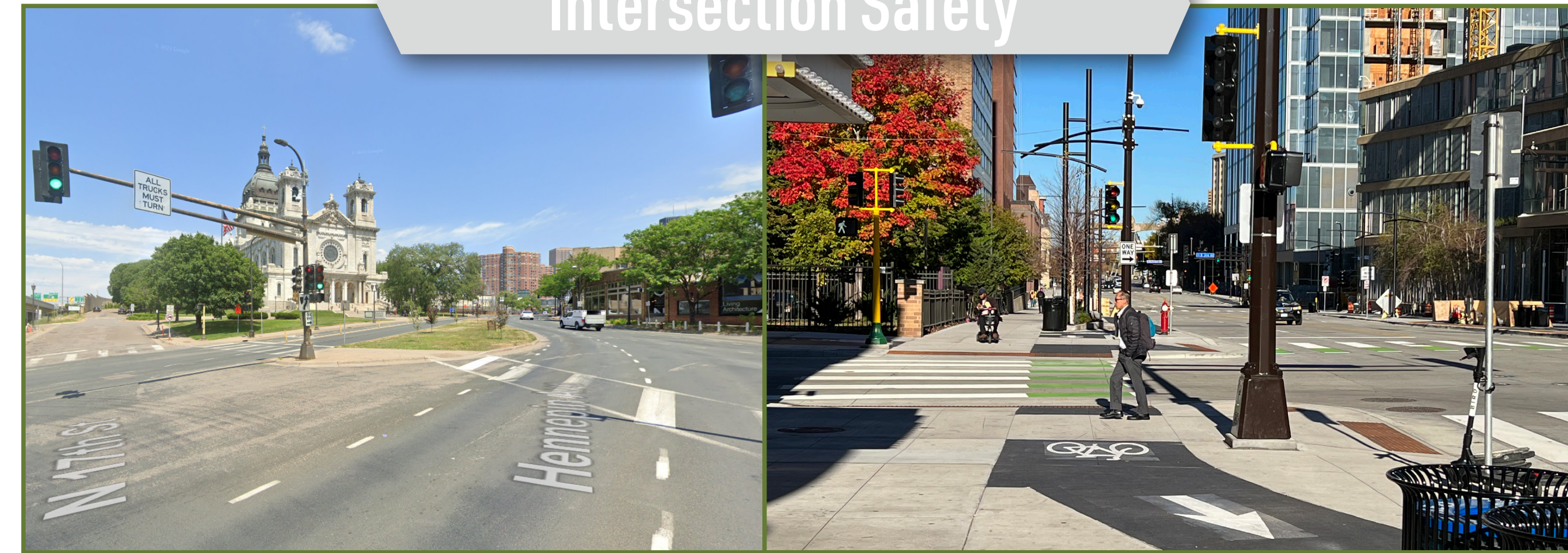
Existing intersection with poor visibility for people walking, ADA ramps, and long crossing distances
