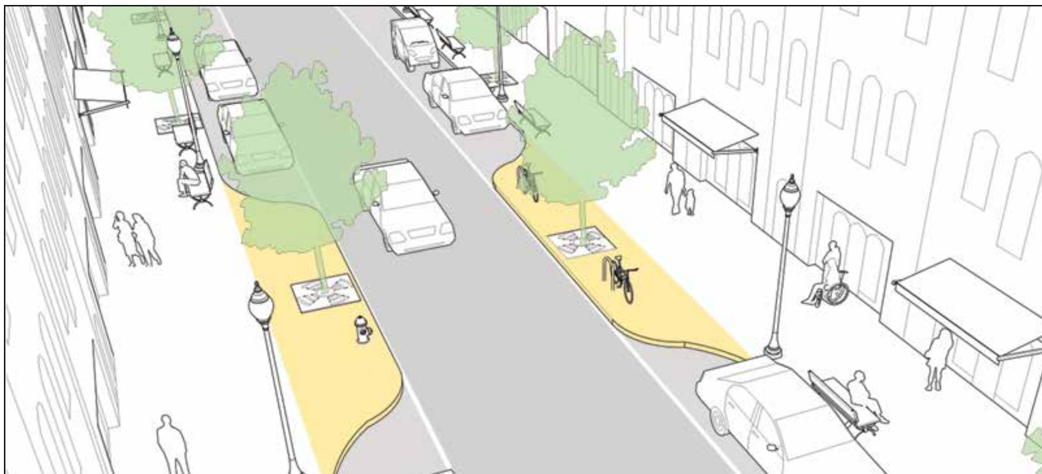
Design treatments to slow speeding cars (example of a "pinchpoint" pictured above. Source: NACTO)
