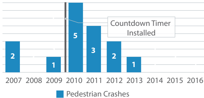
Figure B-31. Before and After Countdown Timers at 1st Ave N and N 4th St
