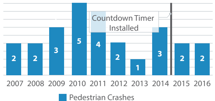
Figure B-34. Before and After Countdown Timers at Franklin Ave and Nicollet Ave
