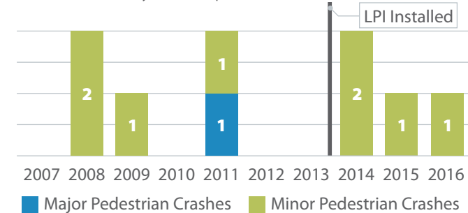
Figure B-15. Before and After LPI Crash Analysis at 4th St SE and 15th Ave SE
