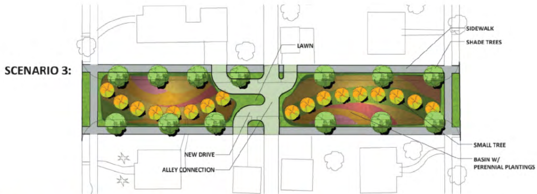
This diagram shows a method of converting a street to a rain garden.
