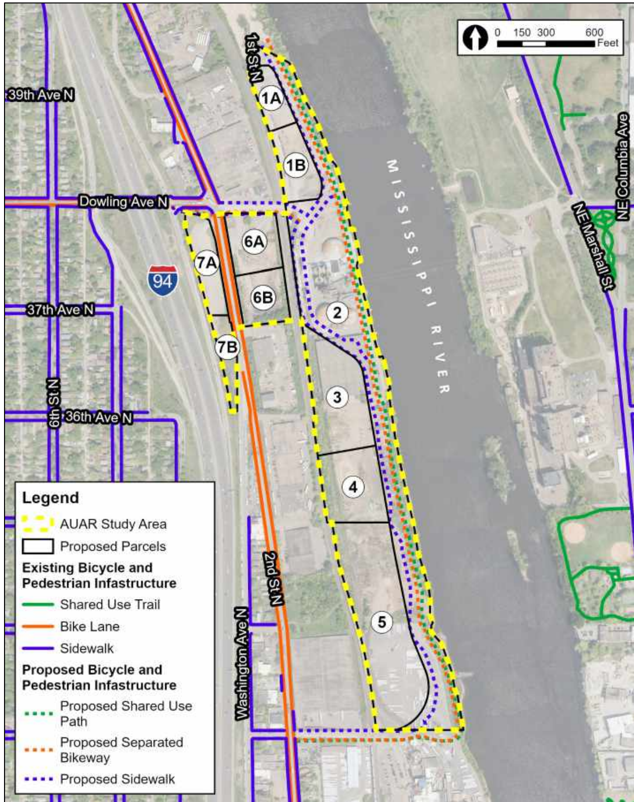
Figure 17: Existing and Proposed Bicycle and Pedestrian Infrastructure
